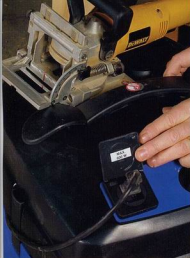
Plug into auto start. A receptacle right on the vacuum will turn the machine on and off in concert with the tool.
