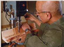
Pocket-hole jig. Construct a small jig to hold the rail at approximately 10^\circ while drilling pocket holes with a Forstner bit.
