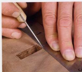
Angle the ends of the mortise. The layout and chopping techniques are the same as when angling a mortise for a single fixed wedge.
