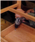
Attached to the tabletop. These fasteners are best fitted to either small tables or to the ends of large tables. They do not allow for much wood movement when fitted perpendicular to the grain of the tabletop.
