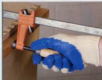
Glove gets good grip. A tight grip comes a lot easier when you wear one of these inexpensive cotton gloves with latex-dipped palms.
