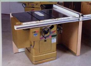
The tables almost disappear. Shop space grows considerably when the extension tables fold down.
