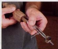
Locate the flame tips. Step off and mark nine equal spaces with dividers at the top.
