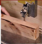
Cut the front curve on the bandsaw. Cut right to the line, then smooth the curve with a block plane and sandpaper.
