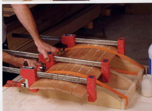
Glue up the panel. Lay the staves on the form to make sure all of the joints close perfectly. Use bar clamps and strap clamps as shown to draw the staves together and down against the form. Use a yellow glue with extended working time.
