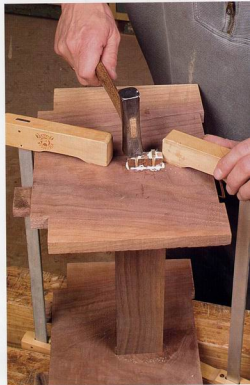
Sometimes clamps are needed. Nessel uses clamps to keep the tenon shoulders snug and square while he drives home the wedges.
