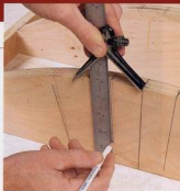
Figure out sections and angles right on the form. Use a center divider to draw lines straight down from each division.
