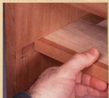
A divider in a stopped dado is inserted from the back. The front rail must be notched to reach the front of the case.
