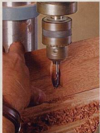
Pocket-hole jig. Construct a small jig to hold the rail at approximately 10^\circ while drilling pocket holes with a Forstner bit.
