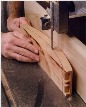
An easy way to cut the inside curve. Lay out the desired curve. Then ride the rip fence as shown to follow that curve, creating a consistent thickness. Use the offset as a sanding block.
