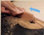
Curved fence to rout a curved groove. After cutting and smoothing the curves in the rails, use the curve template to make a curved fence for the router table. Keep the workpiece steady on the table as you slide it along the fence.
