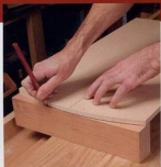
First, lay out the curve. This will determine how deep the dovetails can go.
