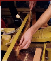
Use a sliding bevel to find the angle for jointing and ripping the staves. Balance the tool on the center of a section as shown to find the angle.
