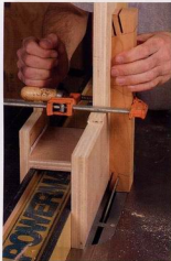
Cut the tenons on the rails while the stock is square. Make the cheek cuts first (left), then make the shoulder cuts (above).
