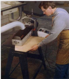
Sander is a time-saver. With an 18-in.-wide drum, the Craftsman tool can sand a workpiece up to 36 in. wide.
